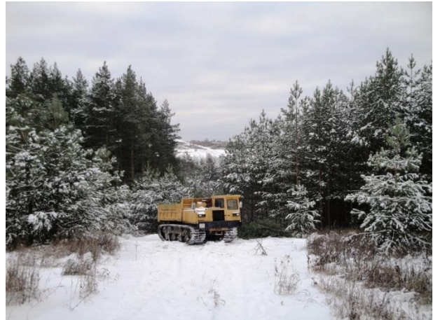
PHOTO No. 6 shows the use of a "Morooka" for transporting soil in difficult circumstances and steep slopes
